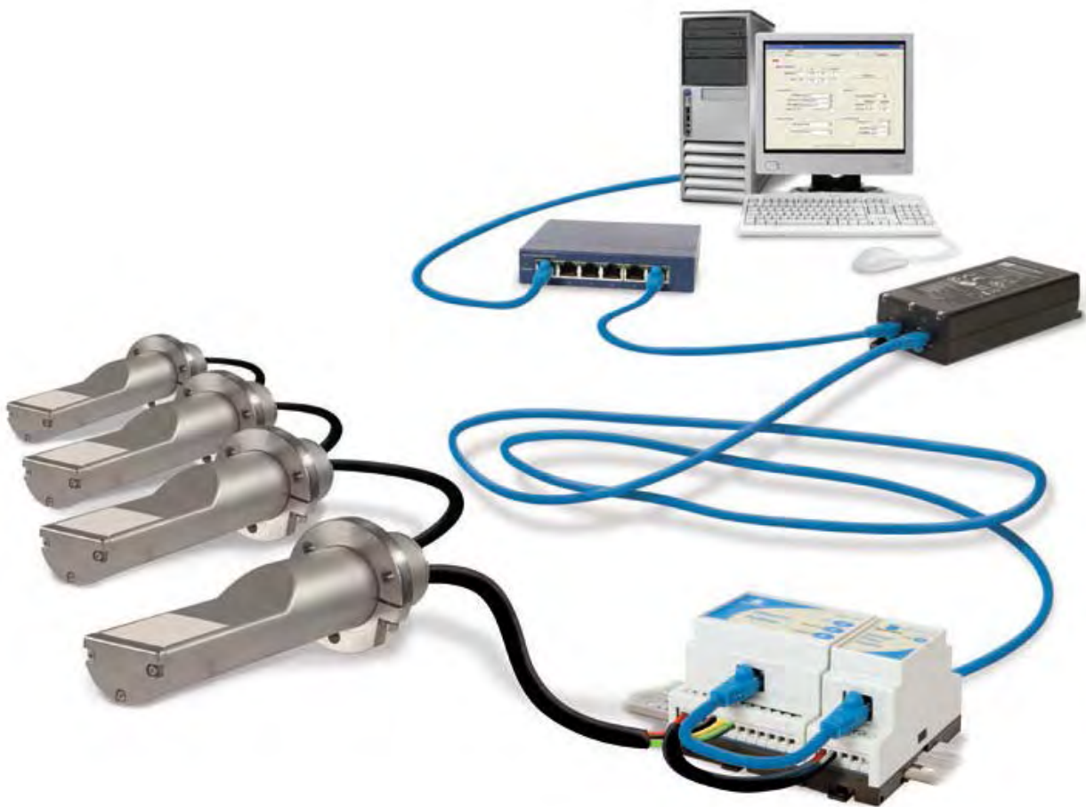
Figure 1: Ethernet Adapter Kit Connections
